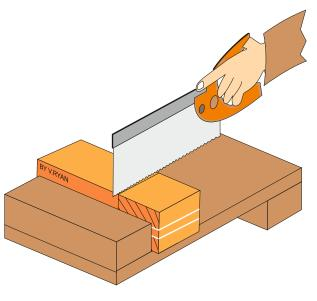
The wood is then supported by a bench hook and a tenon saw is used to finally remove the waste wood. This leaves the shoulder of the joint.
