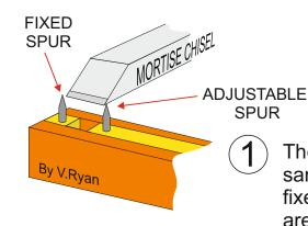
The mortise chisel is carefully selected. It should be the same width as the mortise to be cut into the wood. The fixed spur and the adjustable spur of the mortise gauge are set to the width of the chisel.
