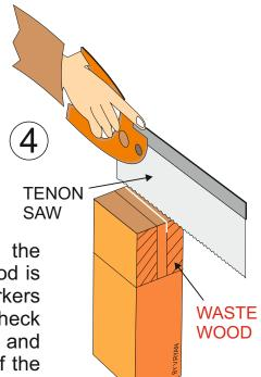
A tenon saw is used saw down the gauged lines of the tenon. The wood is normally held firmly in a woodworkers vice. When sawing, take time to check that the saw is cutting straight down and that it is on the waste wood side of the tenon.
