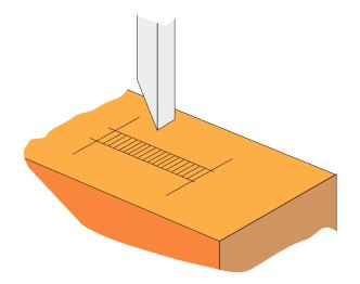
The waste wood is then slowly removed, this time, by applying more force to the handle of the chisel with the mallet. The waste is removed until the entire mortise hole has been cut.
