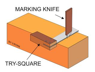
A try square and a marking knife are used mark the lines at the top and bottom of the mortise.
