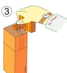
The mortise gauge is used to mark the size of the tenon. The stock of the marking gauge must be held firmly against the side of the wood as wit ill have a tendency to follow the grain of the wood rather than a straight line.
