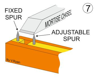
The distance between the fixed spur and the adjustable spur is set so that it matches the width of the mortise chisel. This done by turning the brass thumb screw. The width of the mortise chisel should match the width of the mortise to be cut in the wood.
