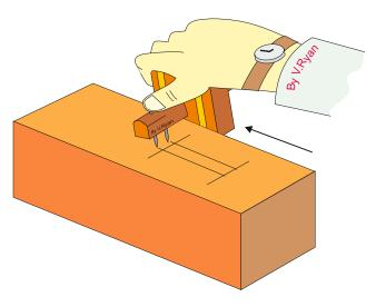
The stock of the mortise gauge is pressed against the side of the wood. It is then pushed along the wood until the mortise is marked out correctly.
